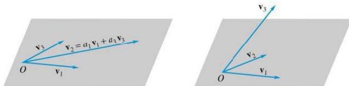
FIGURE 4.26 (a) Linearly dependent vectors in R^3 . (b) Linearly independent vectors in R^3 .
